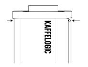
Reinsert the 2 screws removed in step 2. Make sure not to over tighten these. You may need to squeeze the panels together to line up the screw holes.
