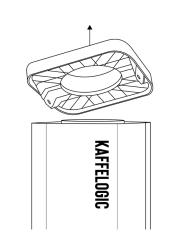
Carefully lift off the top closure making sure not to move the roast chamber. Place the new closure into your unit carefully. Line up the screw holes on the closure with the ones on the panels.
